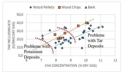
Figure 3.5: Concentration of tar in dry part of the Raw Gas as a function of CH<sub>4</sub> concentration, from [19].
