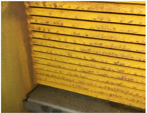
Figure 3.11: Deposits of tar components on the intercoolers in the product gas compressor.
