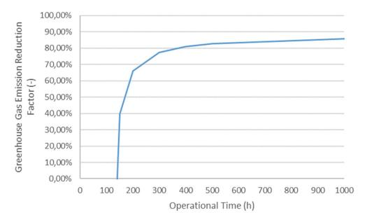
Figure 3.18: Greenhouse gas emission reduction factor as a function of operating time starting from gasification heat-up.
