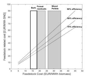
Figure 4.4: Fuel-related costs as a function of fuel costs and moisture content, left, and gasifier efficiency, right. Typical fuel prices in Sweden are indicated by shaded areas. From J. M. Ahlström et al [27].
