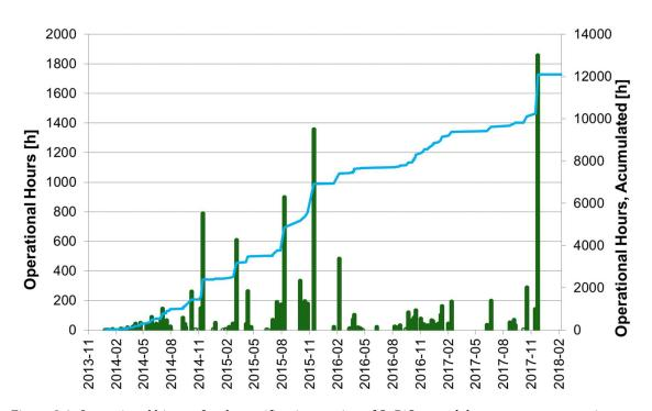
Figure 3.1: Operational history for the gasification section of GoBiGas, each bar represents a continuous run and the line is the accumulated number of operational hours.
