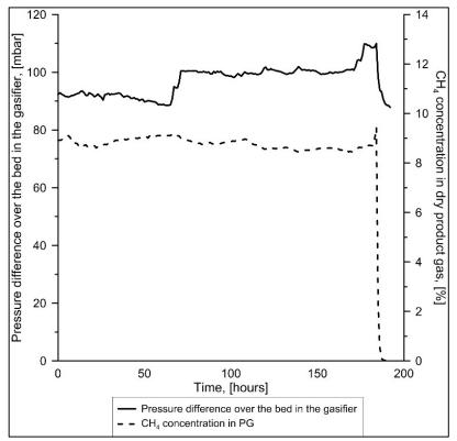
Figure 3.9: Methane concentrations and pressure drops over the gasifier fluidized bed during 200 h of operation as bed height was increased in two steps [15].
