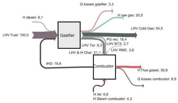
Figure 3.13: Sankey Diagram representing the energy balance of the gasifier section of GoBiGas when operating with wood pellets as fuel (above) and shredded bark with 25% moisture (below), normalized by the energy contents of the fuel based on the lower heating value, see J. M. Ahlström et al [27].
