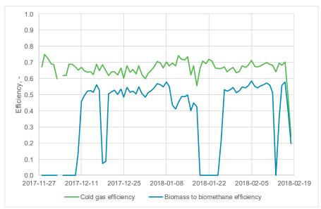
Figure A5.4: Efficiency of the Gasification section (Cold Gas) as well as for the hole process for conversion into biomethane during continuous operation with wood pellets.
