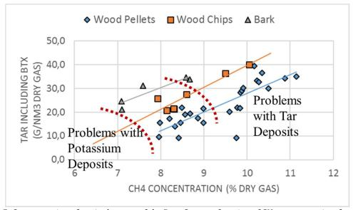
Figure 3.5: Concentration of tar in dry part of the Raw Gas as a function of CH<sub>4</sub> concentration, from [19].
